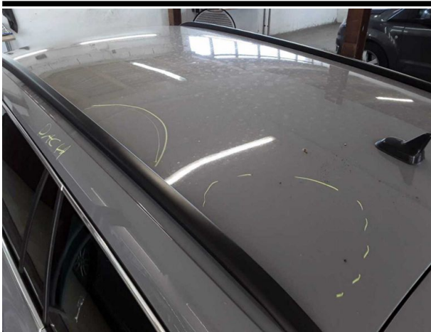
Damage #8: Roof: Roof - dent(s) - Smooth repair work
