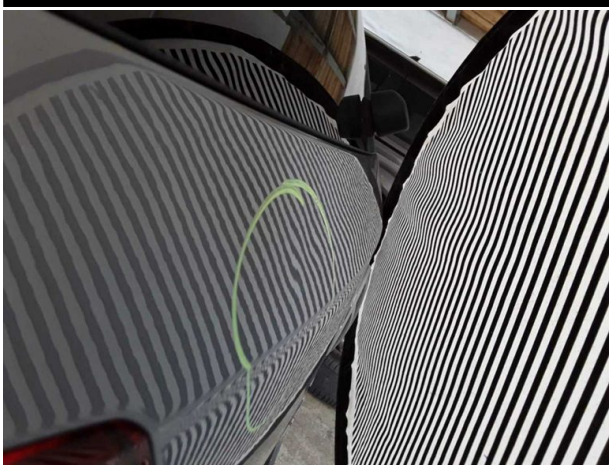
Damage #5: Boot lid / rear door: Boot lid - dent(s) - Smooth repair work
