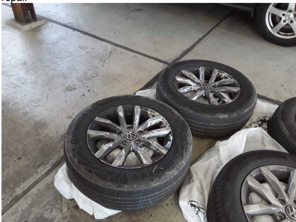
Damage #7: 2nd wheel set: 2 tyres - Worn - Replace
