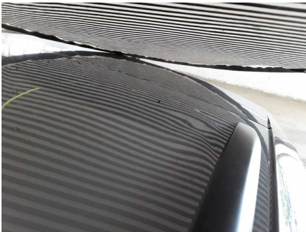
Damage #8: Roof: Roof - dent(s) - Smooth repair work
