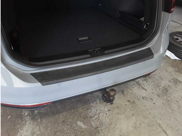
Damage #2: Rear bumper: Rear bumper - Glued / labelled - De-glue / neutralise
