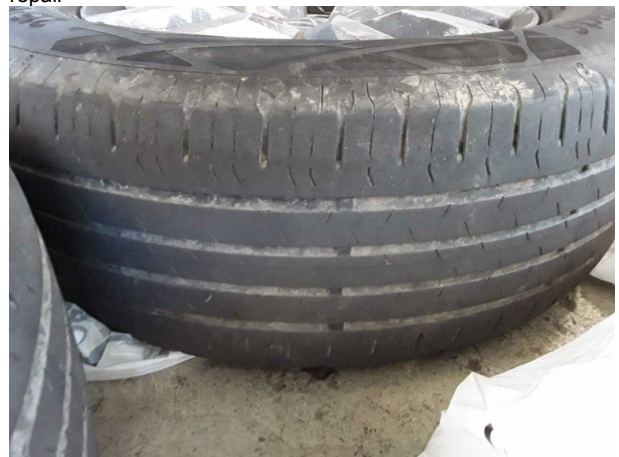
Damage #7: 2nd wheel set: 2 tyres - Worn - Replace
