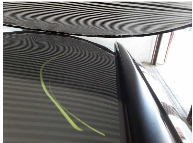
Damage #8: Roof: Roof - dent(s) - Smooth repair work
