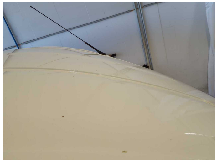
Damage 3: Roof: Roof - dent(s) - Smooth repair work
