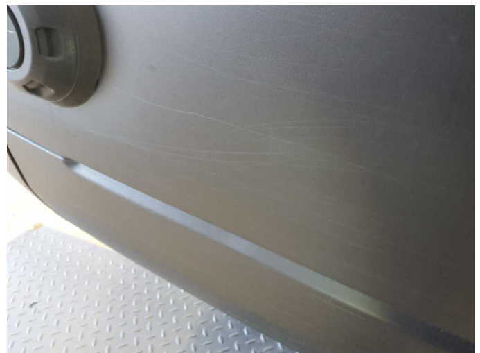
Damage 6: Side panel - rear right side: Brightware - Scratch(es) - Replace
