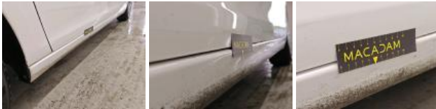
Door RL, Dent(s), Repair and paint (complete)
