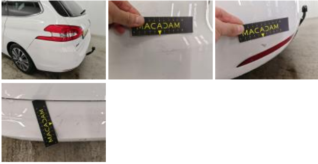
Bumper R, Scratch(es), Repair and paint (complete)
