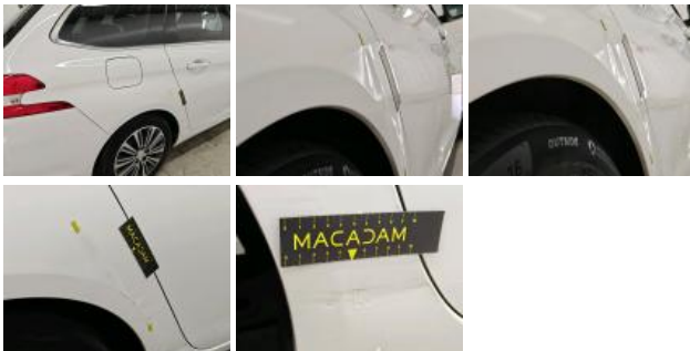
Outer sill R, Dent(s) and scratch(es), Repair and paint (complete)
