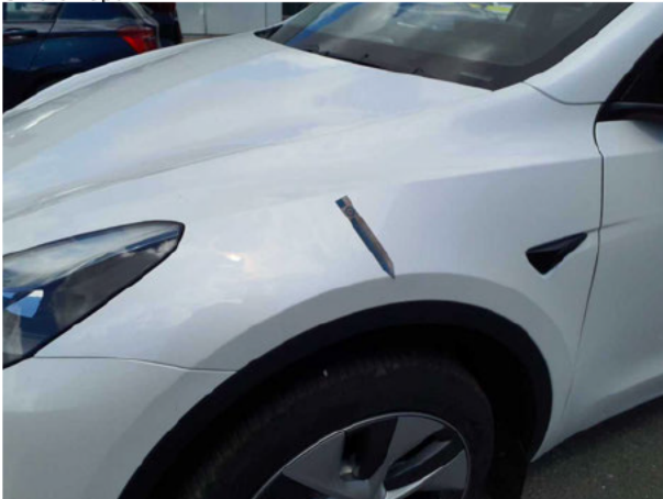
Beschädigung #2: Kotflügel links: Kotflügel links - Delle / Lackschad... - Smart Repair
