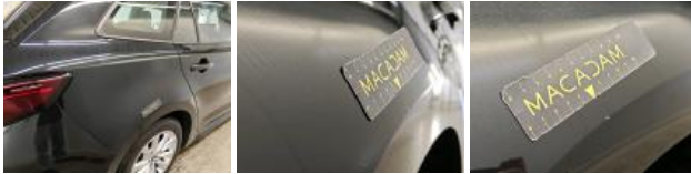
Door FR, Scratch(es), Repair and paint (complete)
