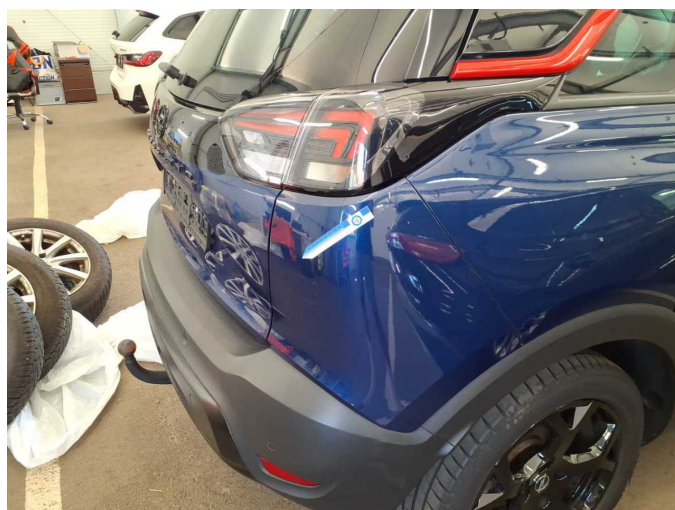
Damage 5: Rear bumper: Bumper - rear right side - Scratched - Paint
