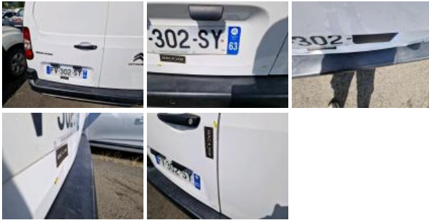
Boot door panel RL, Dent(s) and scratch(es), Repair and paint (complete)
