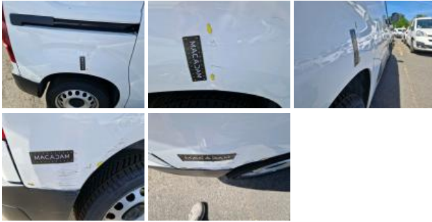
Boot door panel RL, Dent(s) and scratch(es), Repair and paint (complete)
