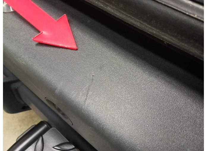
Wear and tear 10: Rear bumper: Rear bumper (Verlade- / Einstiegsbereich) - Scratched - No deduction
