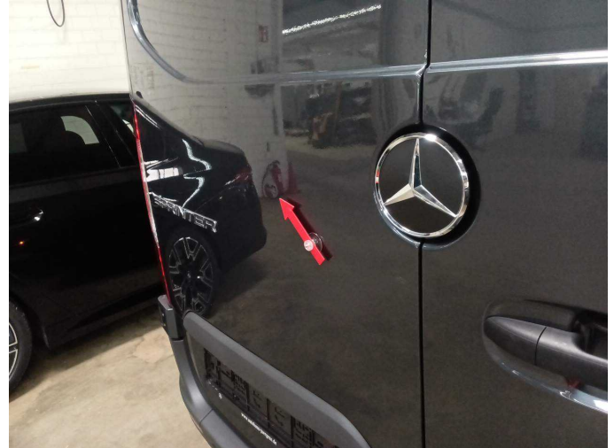
Damage 2: Boot lid / rear door: Rear door - left side - dent(s) - Smart repair
