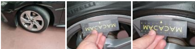
Tyre FL, Worn, Check
