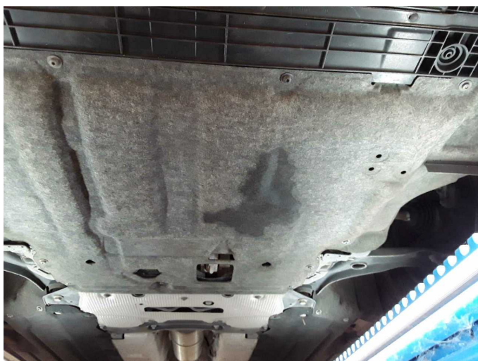
Damage 2: Engine: Engine - Leaking - Perform diagnosis
