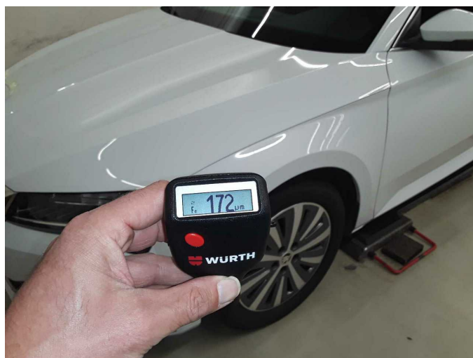
Mudguard - left side: 172 µm
