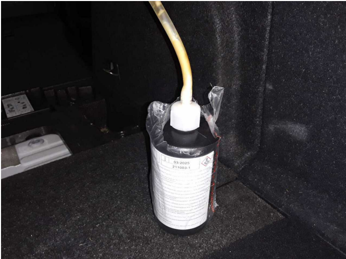
Damage 1: Equipment: Tirefit filler - Empty - Replace
