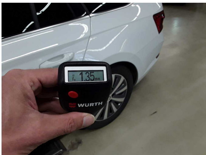
Side panel - rear left side: 1,350 µm
