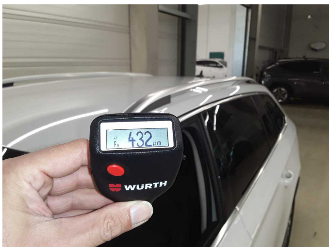
Roof rail - left side: 432 µm
