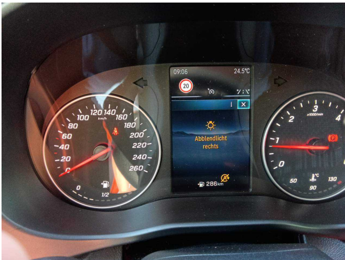
Damage 2: Electrical system: Lighting system (Abblendlicht rechts) - Functional / admissibility - Perform diagnosis
