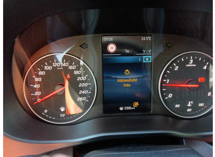
Damage 2: Electrical system: Lighting system (Abblendlicht links) - Functional / admissibility - Perform diagnosis
