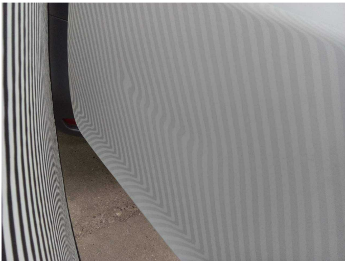
Damage 4: Boot lid / rear door: Rear door - left side (10 cm lang) - dent(s) - Smooth repair work
