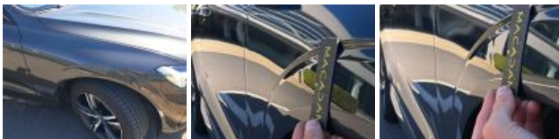
Wing FR, Dent(s), Paintless dent repair
