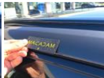
Roof pillar R, Scratch(es), Acceptable
