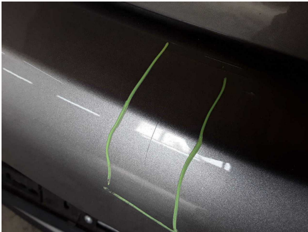
Damage #4: Rear bumper: Rear bumper - Scratched - Paint
