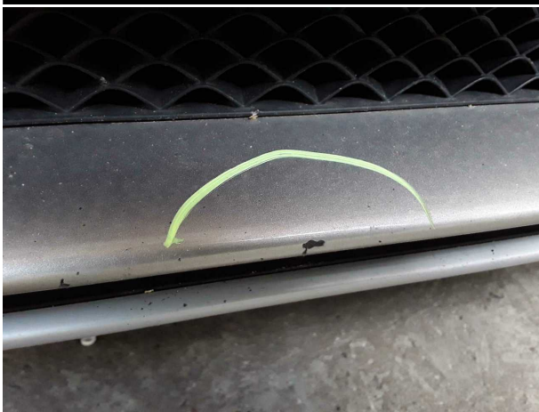
Damage #5: Front bumper: Front bumper - Scratched - Paint
