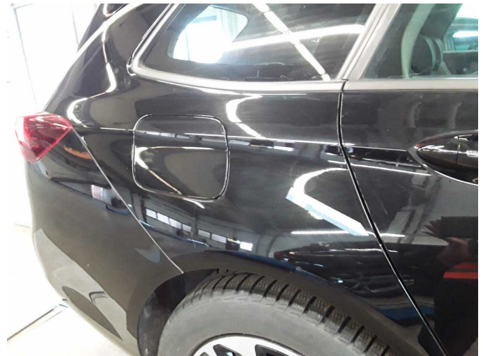
Wear and tear 2: Side panel - rear right side: Side panel - Stone chips - No deduction
