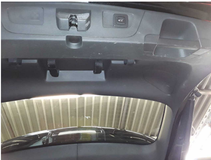
Wear and tear 1: Trim / covers: Boot lid - interior trim - Scratch(es) - No deduction
