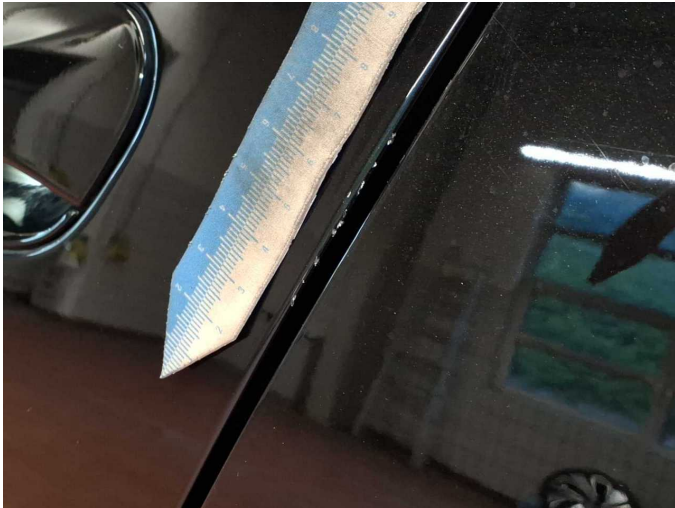
Damage 1: Door - rear left side: Door edge - Scratch(es) - Smart repair
