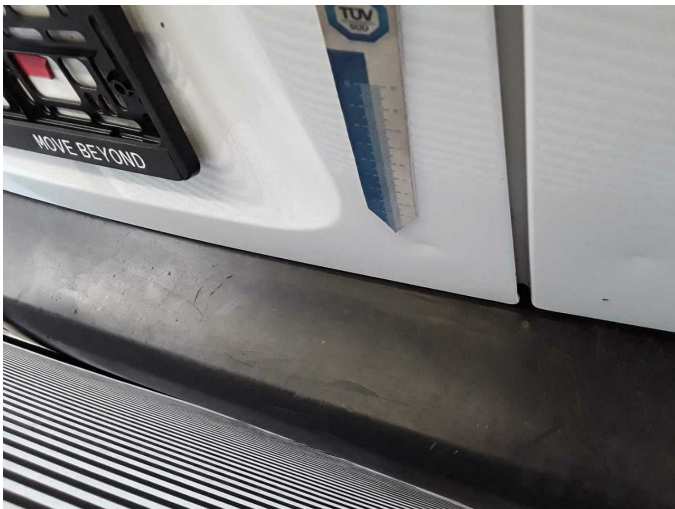
Damage 5: Boot lid / rear door: Rear door - left side - Dent / paintcoat damage - Repair and paint
