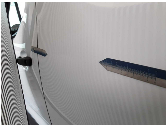
Damage 6: Side panel - rear left side: Side panel - Deformed - Repair and paint
