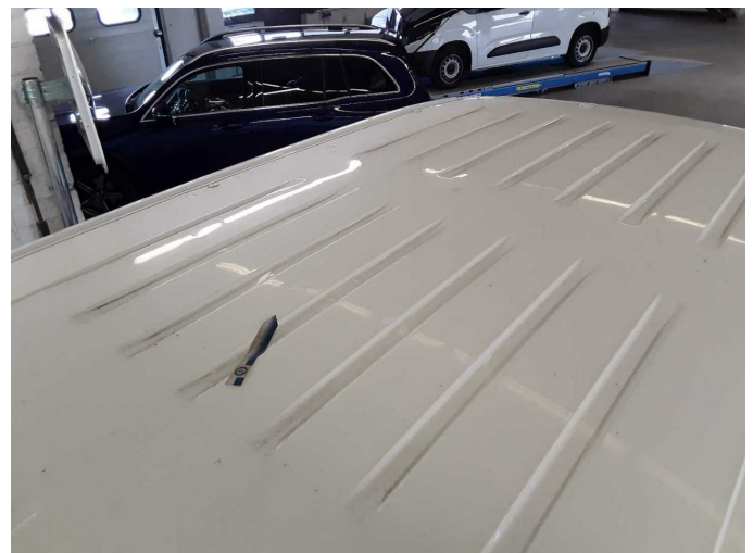
Damage 7: Roof: Roof - Deformed - Repair and paint
