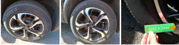
Tyre FL, Out of tolerance, Replace
