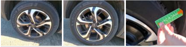
Tyre RL, Out of tolerance, Replace
