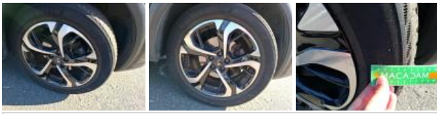
Tyre RR, Out of tolerance, Replace
