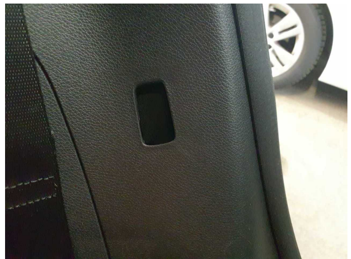
Damage 1: Side panel - rear left side: Sill (Abdeckung) - Loose - Set / adjust
