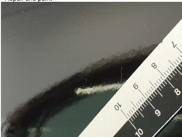
Damage #13: Door - rear left side: Door - Unprofessionally repaired - Repair and paint
