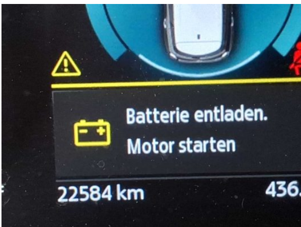
Damage #8: Electrical system: Battery - Functional / admissibility - Perform diagnosis
