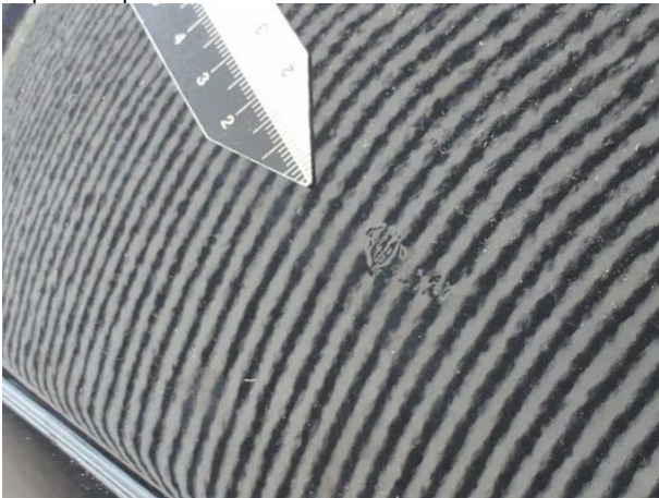
Damage #16: Side panel - rear right side: Side panel - dent(s) - Repair and paint
