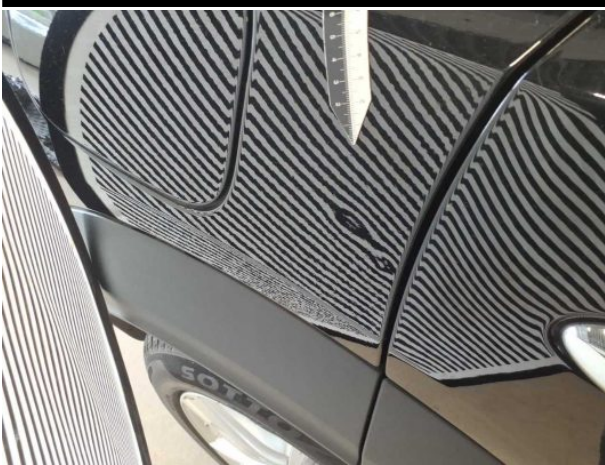
Damage #16: Side panel - rear right side: Side panel - dent(s) - Repair and paint
