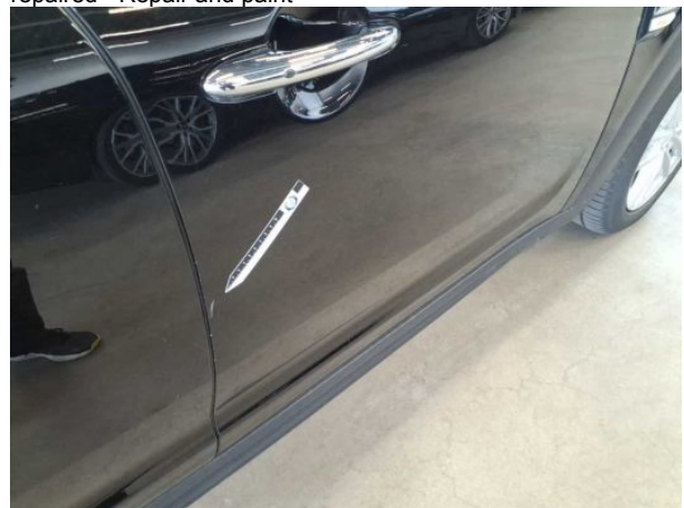
Damage #14: Door - front right side: Door - Scratch(es) - Repair and paint
