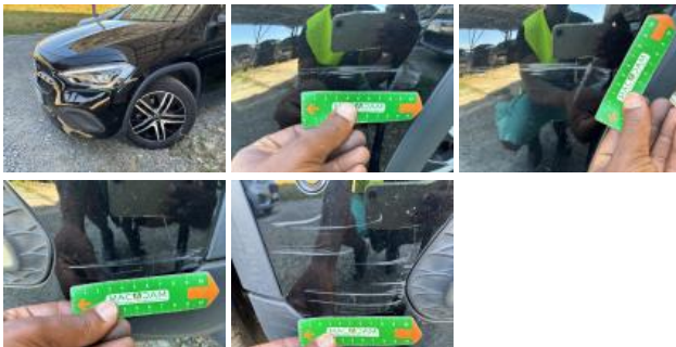
Bumper moulding FR, Scratch(es), Replace
