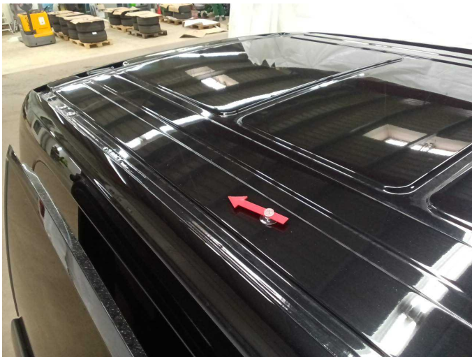
Damage 3: Roof: Roof - dent(s) - Smooth repair work
