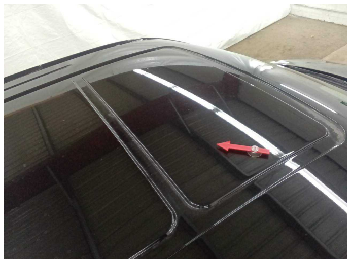
Damage 3: Roof: Roof - dent(s) - Smooth repair work
