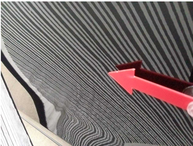
Damage 8: Sliding door - left side: Sliding door - Dent / paintcoat damage - Repair and paint
