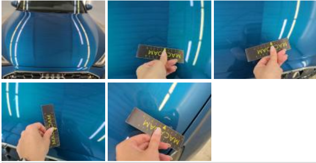
Wing RR, Dent(s), Repair and paint (complete)
