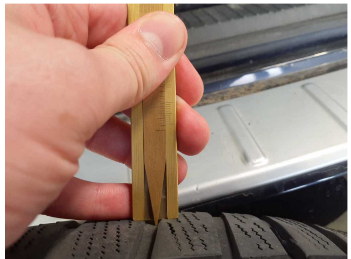
Damage 4: 2nd wheel set: 2 tyres - Worn - Replace
