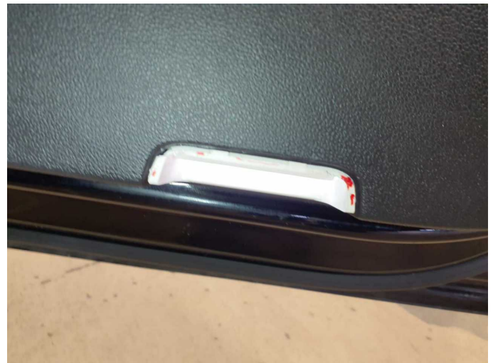
Damage 3: Trim / covers: Trim / covers - Missing - Replace
