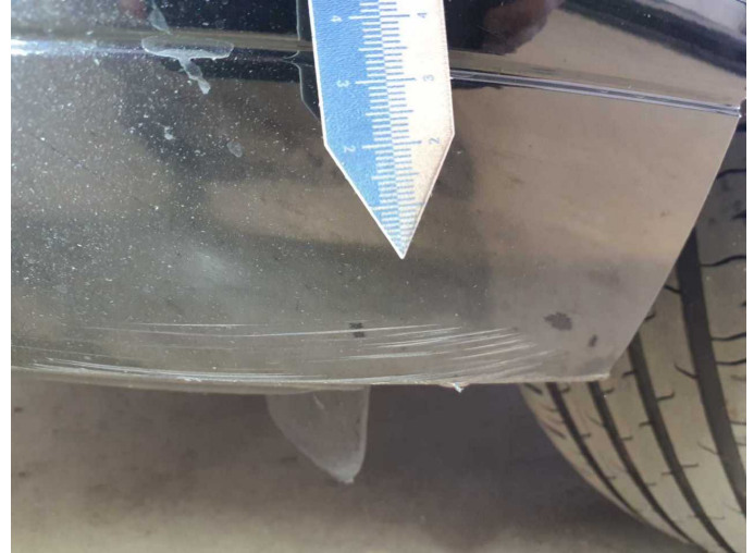
Damage 8: Front bumper: Front bumper - Scratch(es) - Paint
