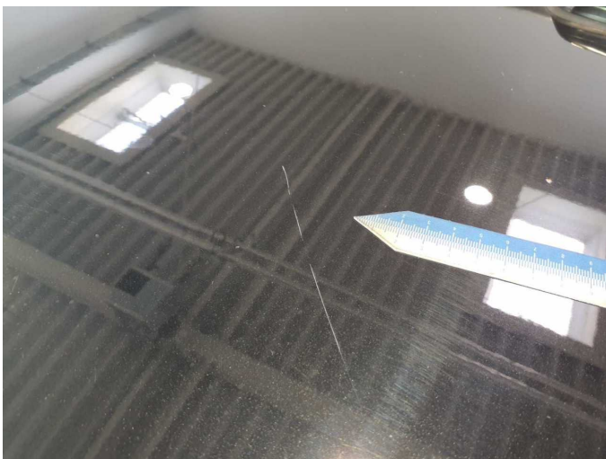
Damage 9: Roof: Roof - Scratch(es) - Paint
