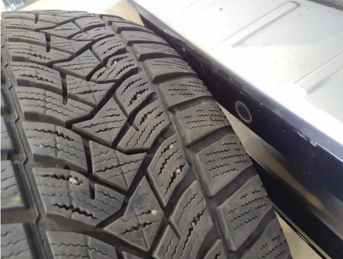
Damage 4: 2nd wheel set: 2 tyres - Worn - Replace
