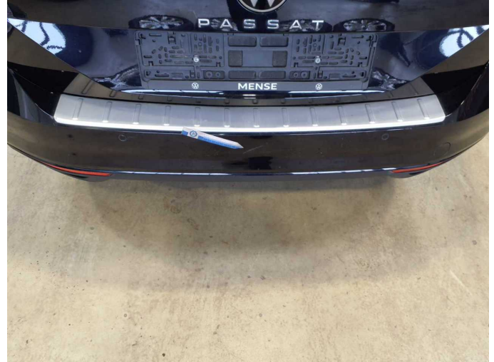
Damage 7: Rear bumper: Rear bumper - Scratch(es) - Paint
