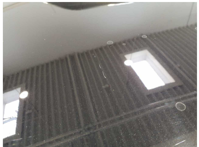
Damage 9: Roof: Roof - Scratch(es) - Paint
