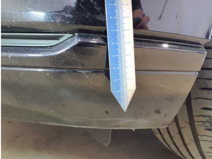
Damage 8: Front bumper: Front bumper - Scratch(es) - Paint
