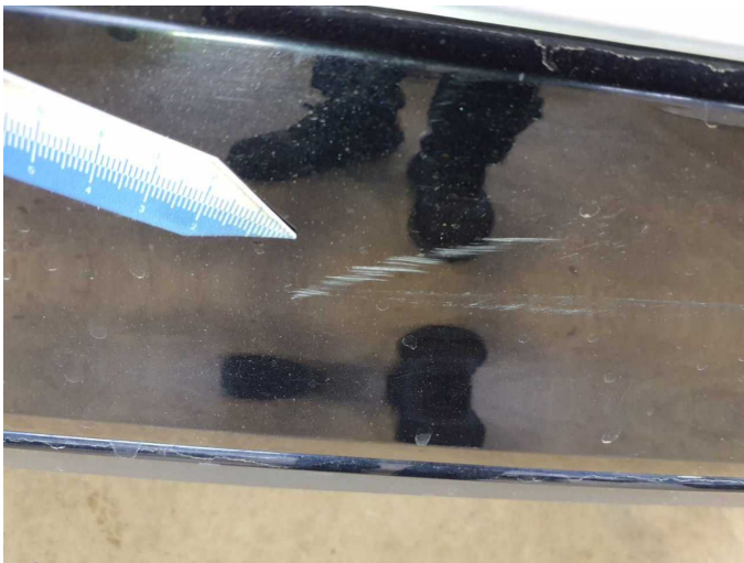
Damage 7: Rear bumper: Rear bumper - Scratch(es) - Paint
