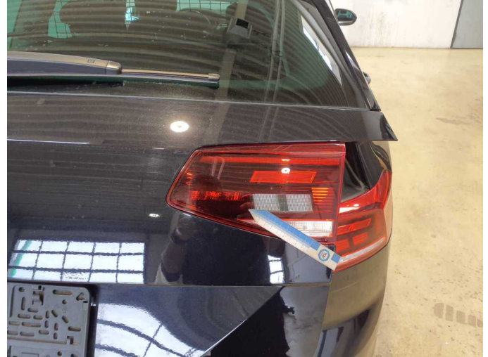
Damage 5: Tail light: Tail lamp - right side - Broken / torn - Replace
