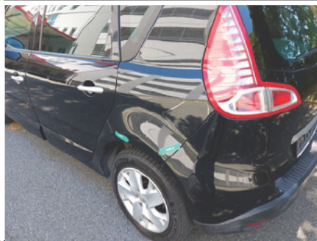
Kotflügel / Hinten Links / Delle
