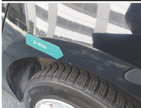
Kotflügel / Hinten Links / Delle
