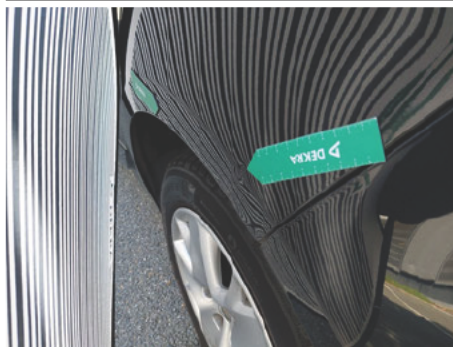
Kotflügel / Hinten Links / Delle
