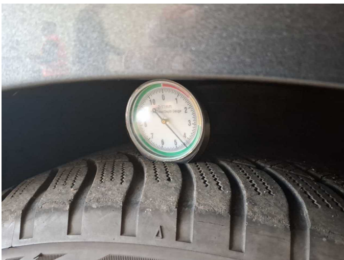
Wear and tear 6: Wheel / tyres: Tyre - front left side - Abrasion - No deduction
