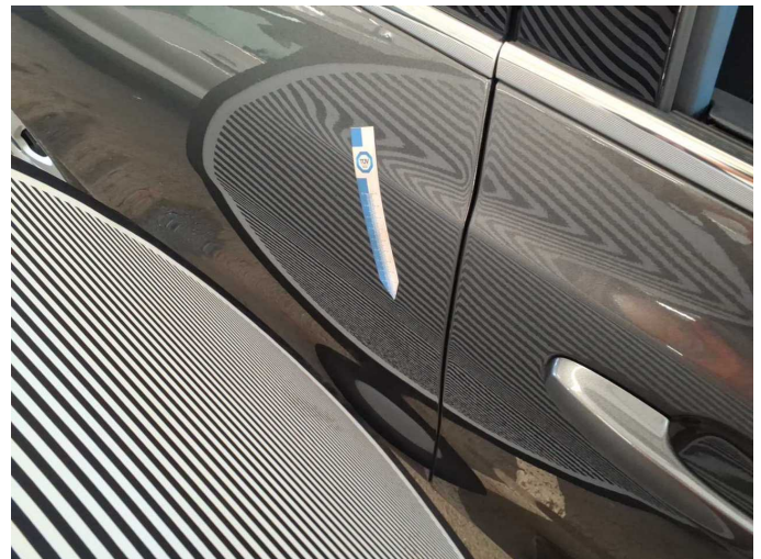
Wear and tear 5: Door - rear right side: Door - dent(s) - No deduction
