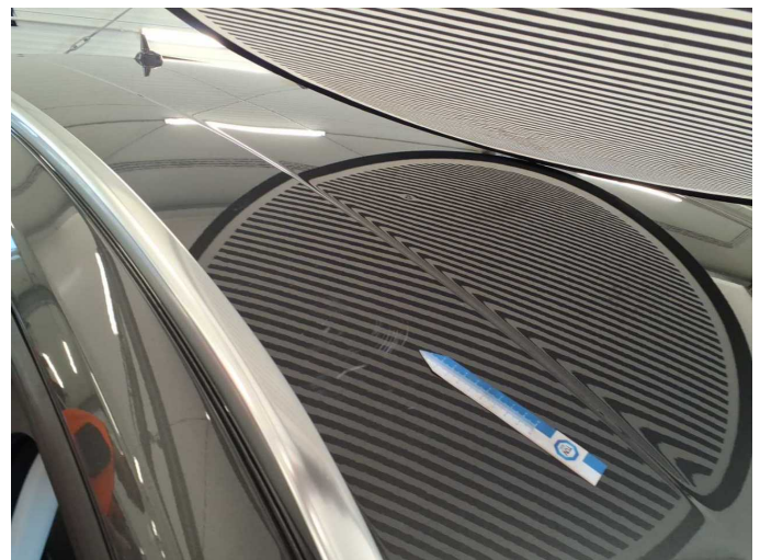
Damage 10: Roof: Roof - Dent / paintcoat damage - Repair and paint
