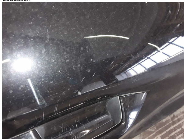
Damage #3: Door - rear right side: Door - Scratched - Cover / polish
