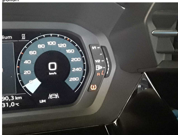
Damage #5: Instrument panel: Indicator light (Riefendruck) - Specify findings - Diagnosed and repair if necessary
