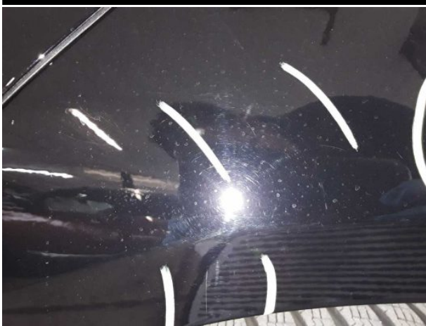
Damage #10: Side panel - rear left side: Side panel - Dent / paintcoat damage - Repair and paint
