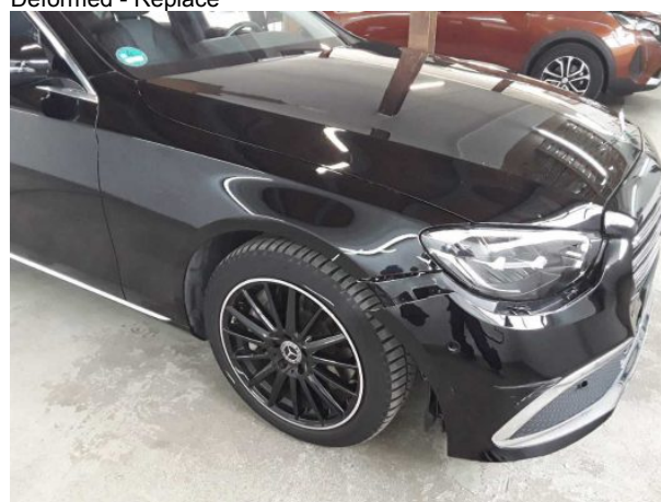
Damage #8: Mudguard - right side: Mudguard - right side - Deformed - Repair and paint
