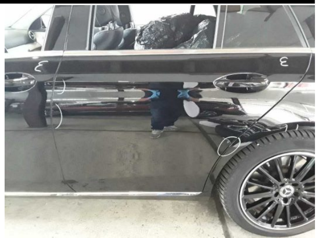
Damage #9: Door - rear left side: Door - Scratched - Paint
