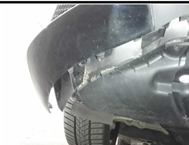
Damage #4: Body: Underbody panelling - Broken / torn - Replace
