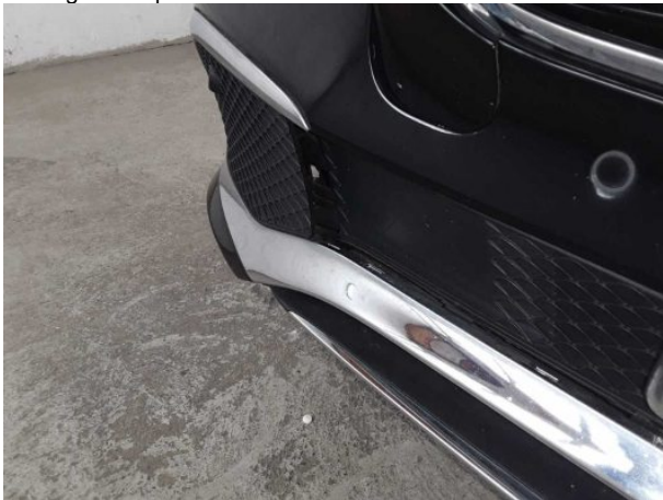
Damage #11: Front bumper: Bumper with Parktronic (Laut Ga.) - Damaged - Replace
