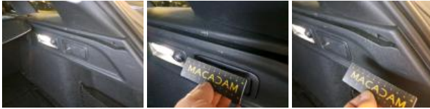
Internal boot lining L, Scratch(es), Acceptable
