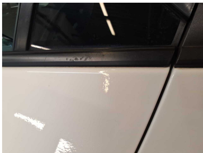
Damage 5: Door - rear left side: Door (Lackpickel) - Unprofessionally repaired - Paint
