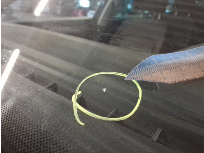
Damage 9: Vehicle glazing: Windscreen (Sichtfeld) - Stone chips - Replace
