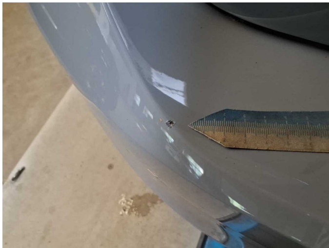
Damage 8: Rear bumper: Rear bumper - Scratched - Paint
