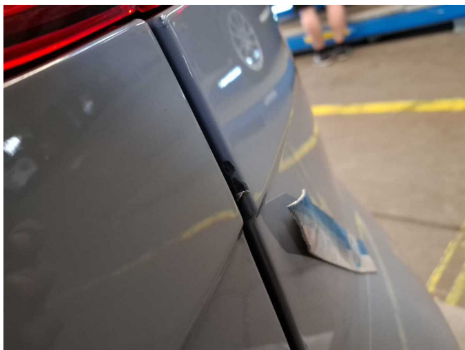
Damage 8: Rear bumper: Rear bumper - Scratched - Paint
