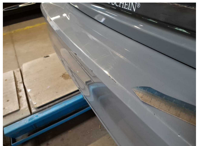
Damage 8: Rear bumper: Rear bumper - Scratched - Paint
