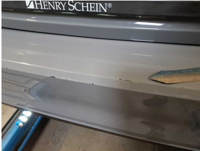
Damage 8: Rear bumper: Rear bumper - Scratched - Paint
