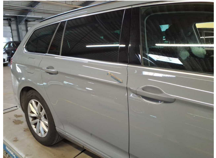
Damage 7: Door - rear right side: Door - Dent / paintcoat damage - Paint
