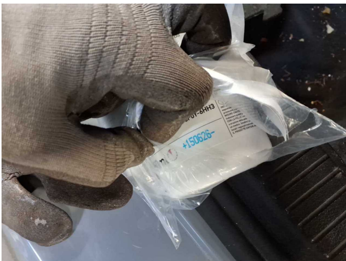
Damage 1: Equipment: Tirefit filler - Expired - Replace
