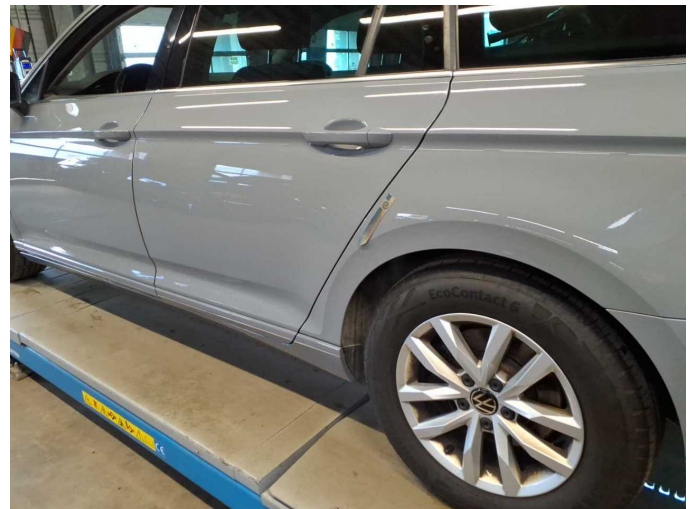
Damage 4: Side panel - rear left side: Side panel - dent(s) - Smart repair
