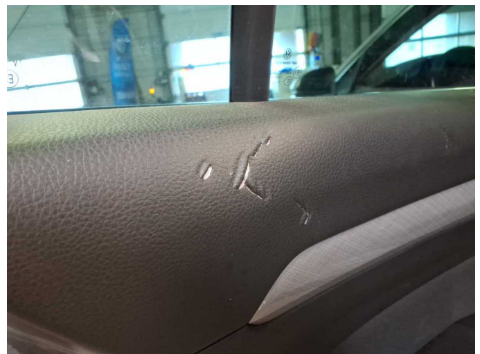
Damage 6: Trim / covers: Door trim - rear left side - Broken / torn - Replace
