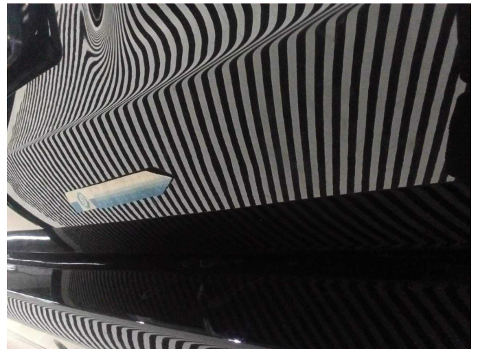
Wear and tear 3: Boot lid / rear door: Boot lid (2 Dellen) - dent(s) - No deduction
