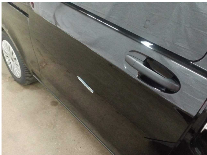
Wear and tear 4: Sliding door, right: Sliding door - dent(s) - No deduction
