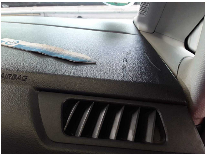
Damage 7: Instrument panel: Centre console - front - Scratched - Smart repair
