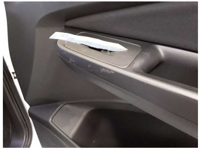
Damage 2: Trim / covers: Door trim - front right side - Scratched - Smart repair
