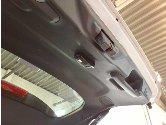
Damage 3: Trim / covers: Boot lid - interior trim (Alarmanlage) - Differs from the original configuration - Replace
