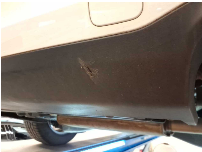
Damage 4: Rear bumper: Spoiler - Broken / torn - Replace
