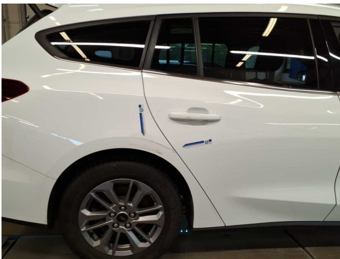
Damage 1: Door - rear right side: Door handle - outside - Scratch(es) - Smart repair
