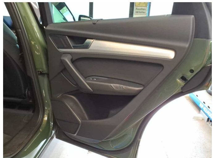
Damage 4: Trim / covers: Door trim - rear right side - Deformed - Smart repair
