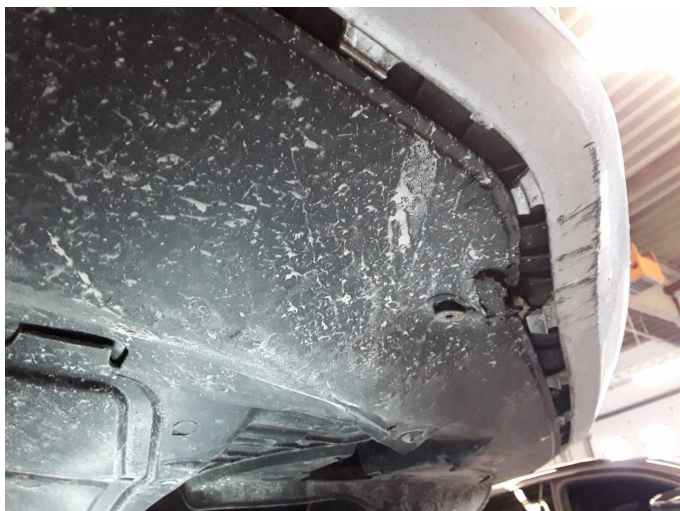
Damage 1: Body: Underbody panelling - Broken / torn - Replace
