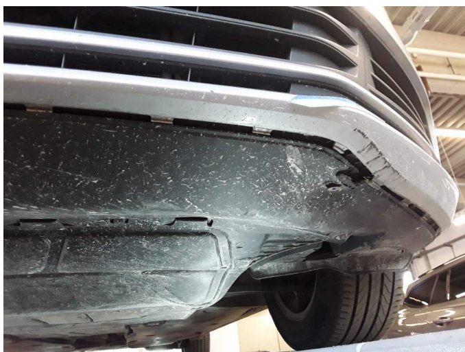
Damage 1: Body: Underbody panelling - Broken / torn - Replace
