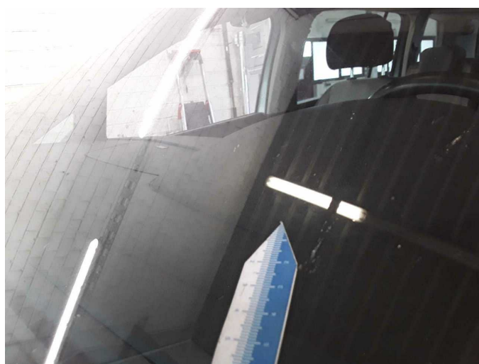
Wear and tear 3: Vehicle glazing: Windscreen - Stone chips - No deduction
