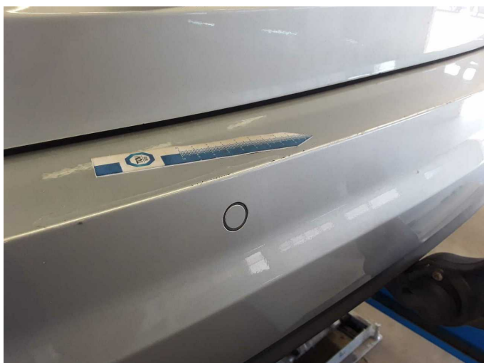
Damage 2: Rear bumper: Rear bumper - Scratch(es) - Paint
