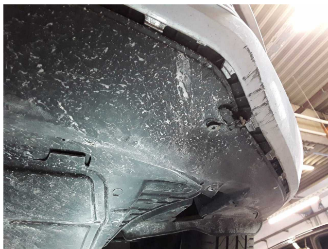
Damage 1: Body: Underbody panelling - Broken / torn - Replace
