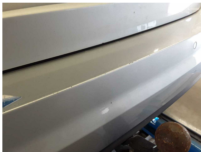
Damage 2: Rear bumper: Rear bumper - Scratch(es) - Paint
