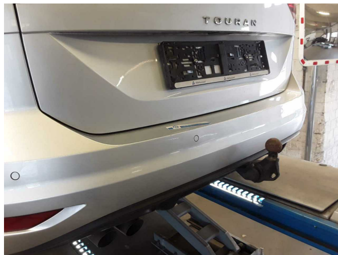
Damage 2: Rear bumper: Rear bumper - Scratch(es) - Paint
