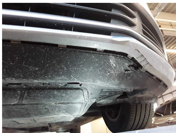
Damage 4: Front bumper: Front bumper - Damaged - repair according to calculation
