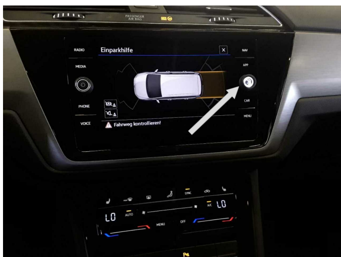
Damage 3: Multimedia system: Screen (Knopf) - Damaged - Replace
