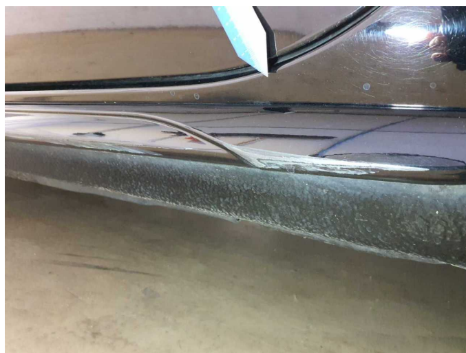
Damage 7: Sill - left side: Trim - Scratch(es) - Replace
