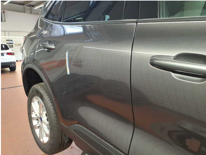
Damage 2: Door - rear right side: Door - dent(s) - Smooth repair work
