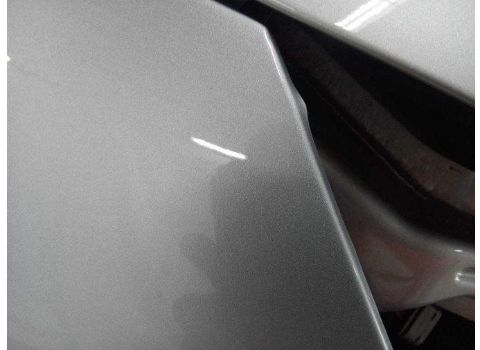
Damage 5: Mudguard - right side: Mudguard - right side - Deformed - Repair and paint
