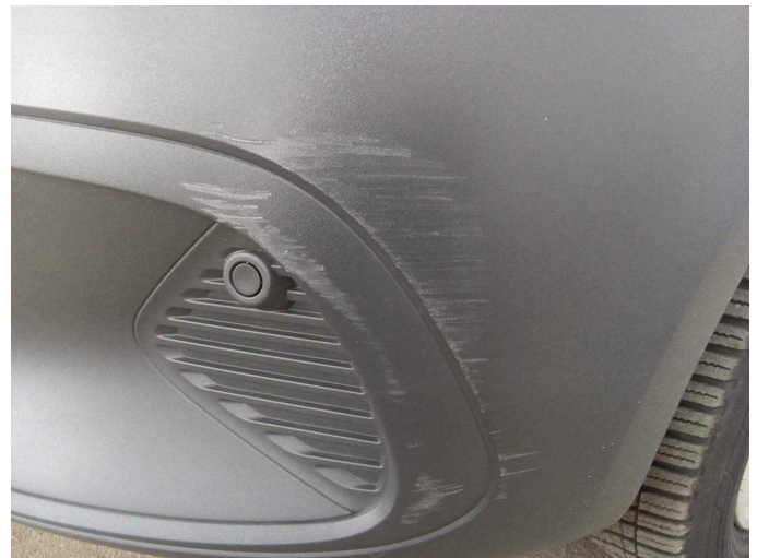
Damage 4: Front bumper: Front bumper - Scratch(es) - Replace
