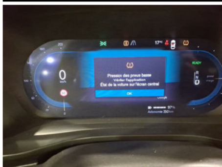
Bandenspanning indicator / Defect
