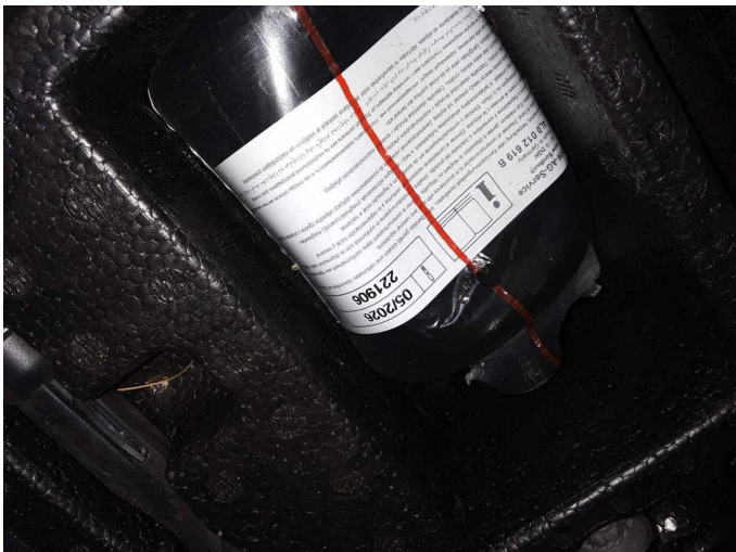
Damage 2: Equipment: Tirefit filler - Due - Replace
