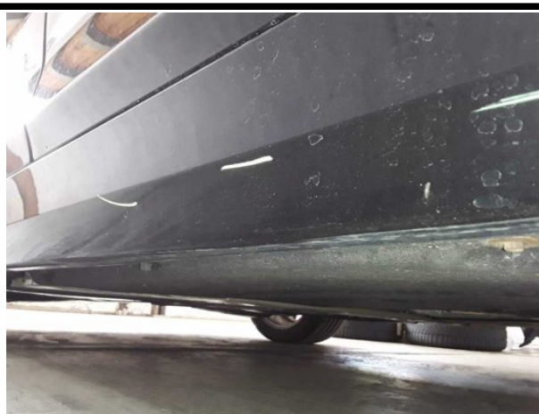
Damage #6: Sill - right side: Trim - Scratched - Repair and paint
