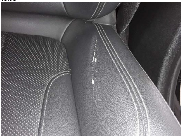
Damage #4: Seat - front: Seat cover - left side - Broken / torn - Replace
