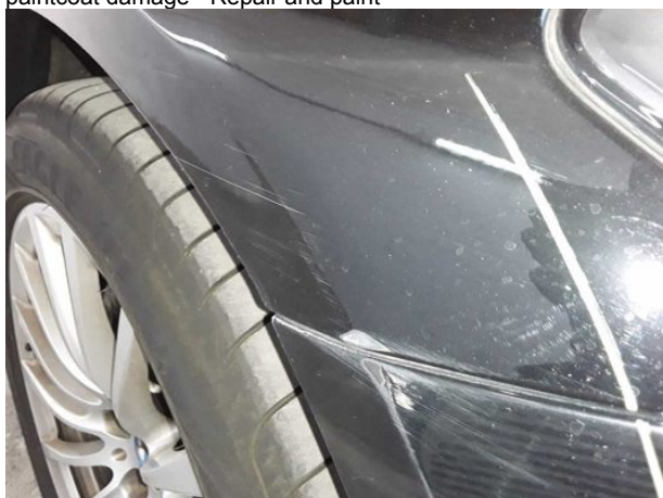
Damage #7: Mudguard - right side: Mudguard - right side - Dent / paintcoat damage - Repair and paint
