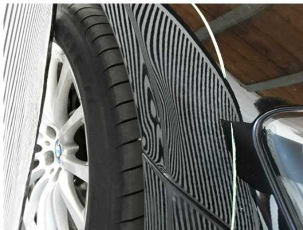
Damage #7: Mudguard - right side: Mudguard - right side - Dent / paintcoat damage - Repair and paint
