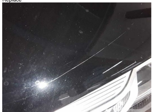
Damage #10: Bonnet: Bonnet - Scratched - Repair and paint
