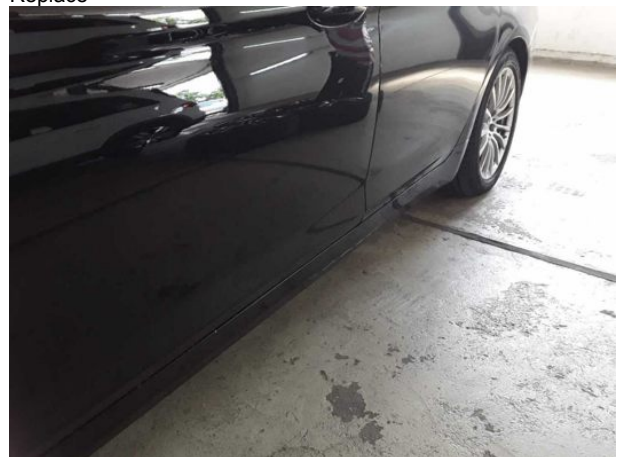
Damage #5: Sill - left side: Trim - Scratched - Repair and paint
