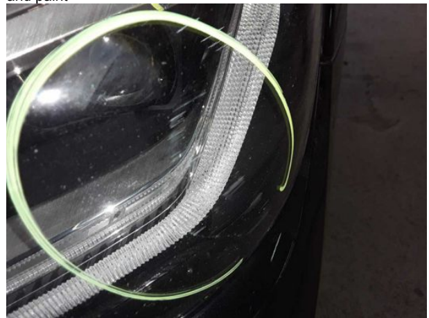
Damage #9: Headlight: LED headlight left - Scratched - Replace
