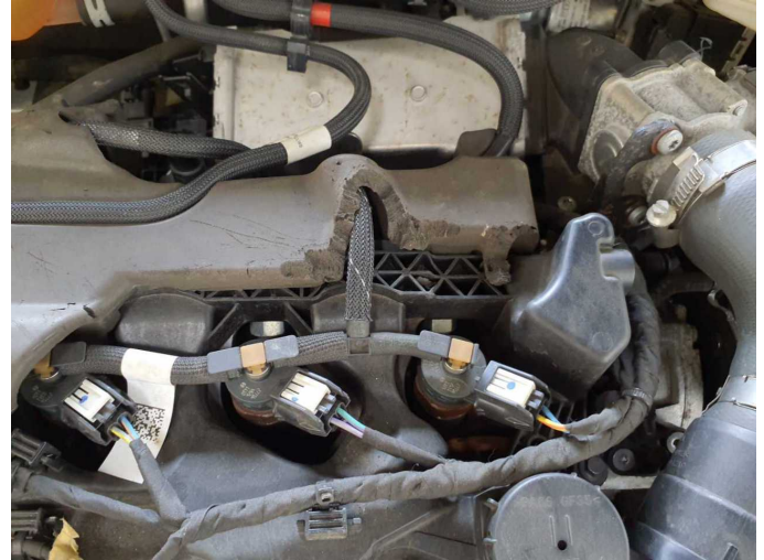
Damage 5: Engine: Engine cover - Damaged - Replace
