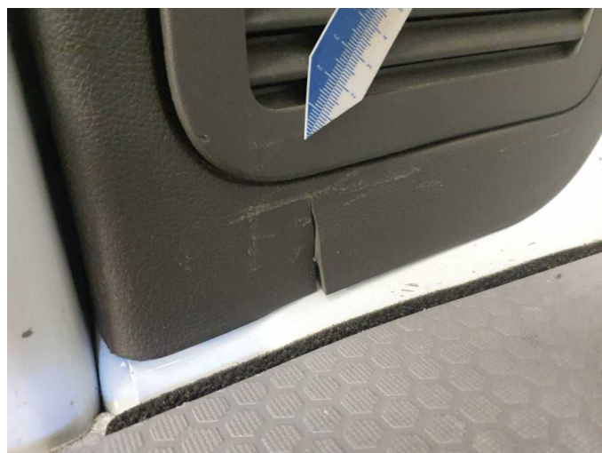
Damage 4: Trim / covers: Cargo area - lining -left side - Broken / torn - Replace
