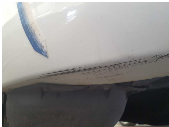
Damage 5: Front bumper: Front bumper - Scratch(es) - Paint
