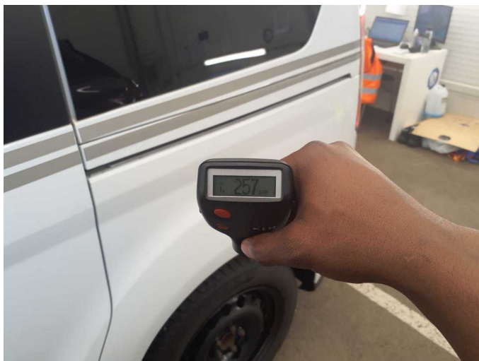
Repainting 1: Side panel - rear left side
