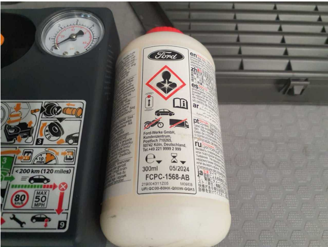
Damage 1: Equipment: Tirefit filler - Expired - Replace
