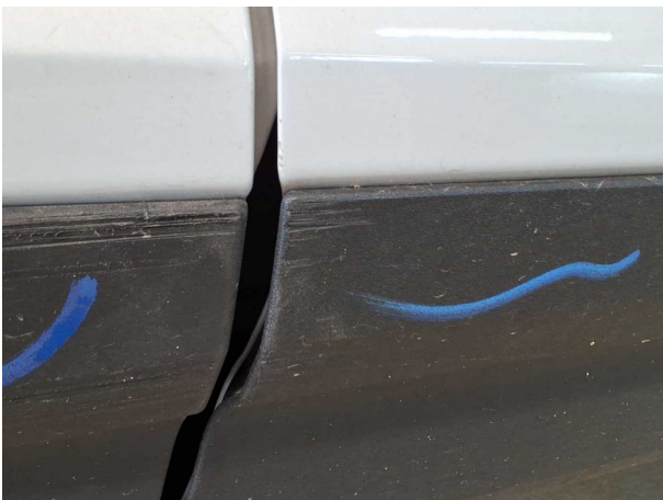
Damage #3: Door - front right side: Brightware - lower - Scratched... Replace
