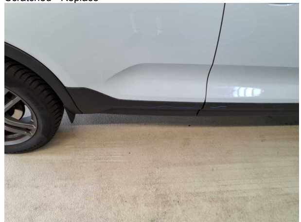
Damage #4: Door - rear right side: Brightware - lower - Scratched - Replace
