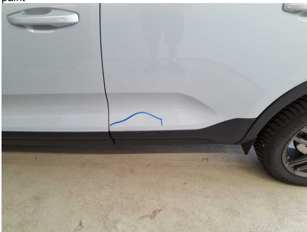
Damage #7: Door - rear left side: Door - Scratched - Repair and paint
