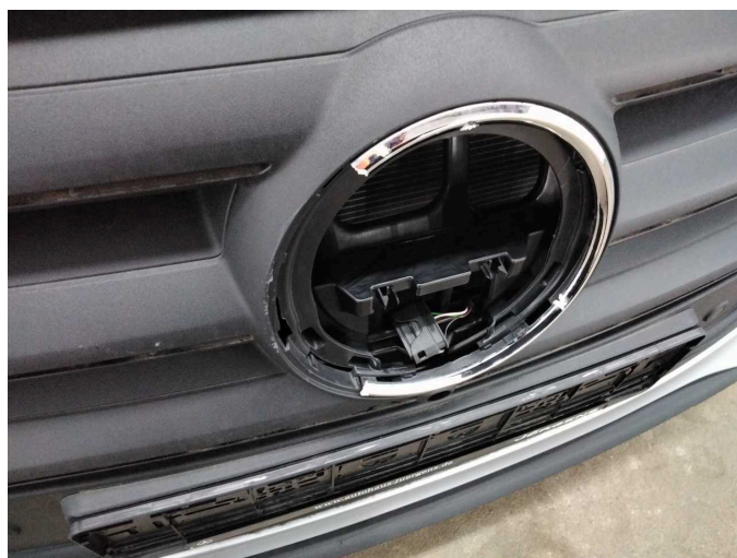
Damage 3: Bonnet: Radiator grille (Emblem) - Broken / torn - Replace
