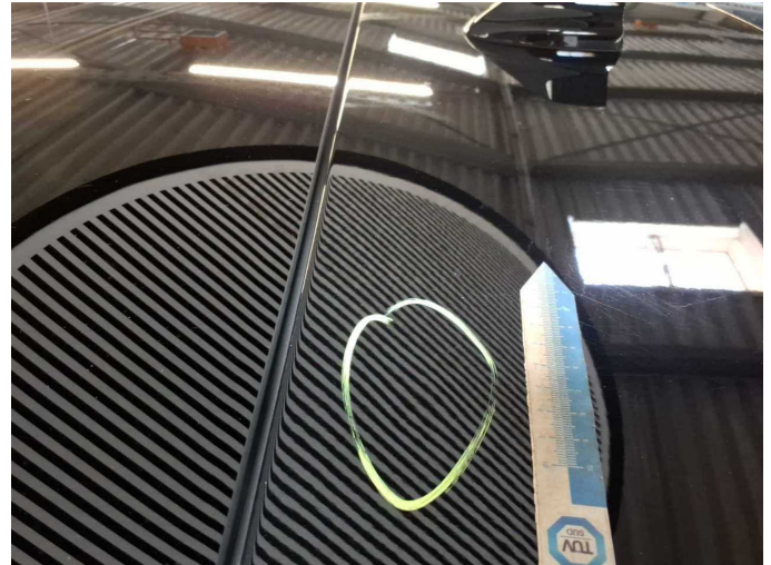
Damage 4: Roof: Roof - dent(s) - Smooth repair work
