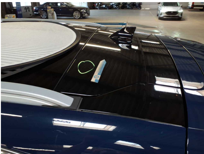
Damage 4: Roof: Roof - dent(s) - Smooth repair work
