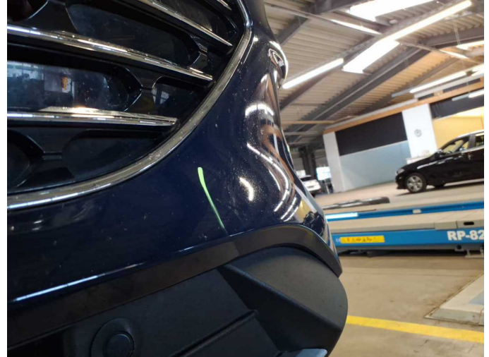
Damage 11: Front bumper: Front bumper (Sandstrahleffekt) - Stone chips - Paint
