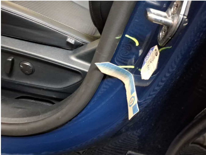
Damage 3: Body: B-pillar - left side - dent(s) - Smooth repair work
