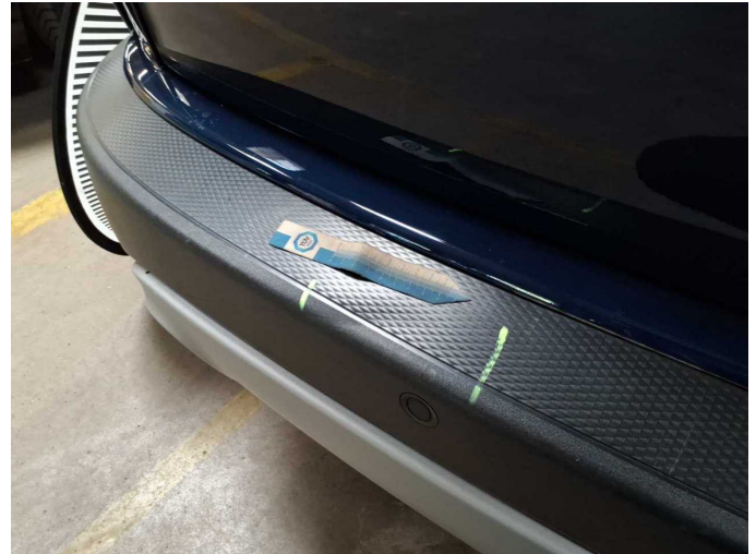
Damage 9: Rear bumper: Rear bumper (unpainted) - dent(s) - Loss in value
