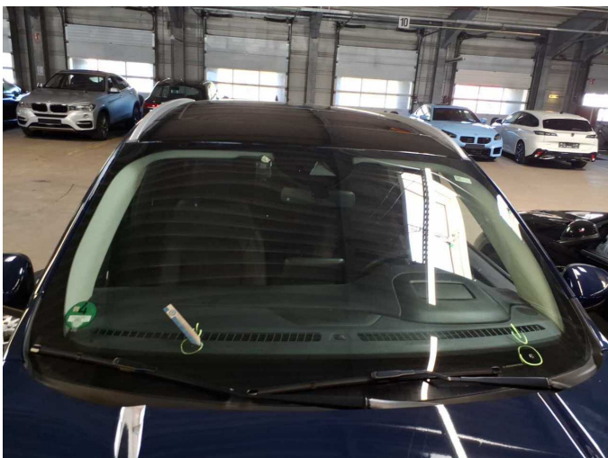
Damage 13: Vehicle glazing: Windscreen - Stone chips - repair according to calculation
