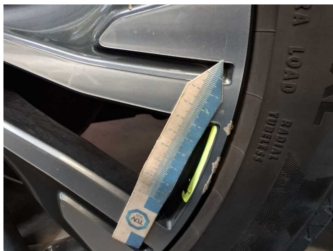
Wear and tear 3: Wheel / tyres: Alloy rim - rear right side - Scratch(es)
