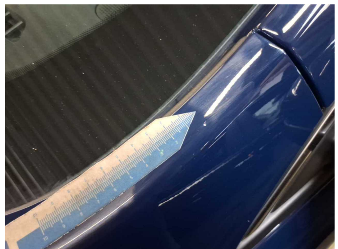
Damage 7: Mudguard - left side: Mudguard - left side - Stone chips - Smart repair
