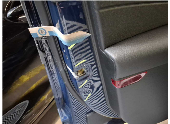
Damage 6: Door - front left side: Door - dent(s) - Smooth repair work
