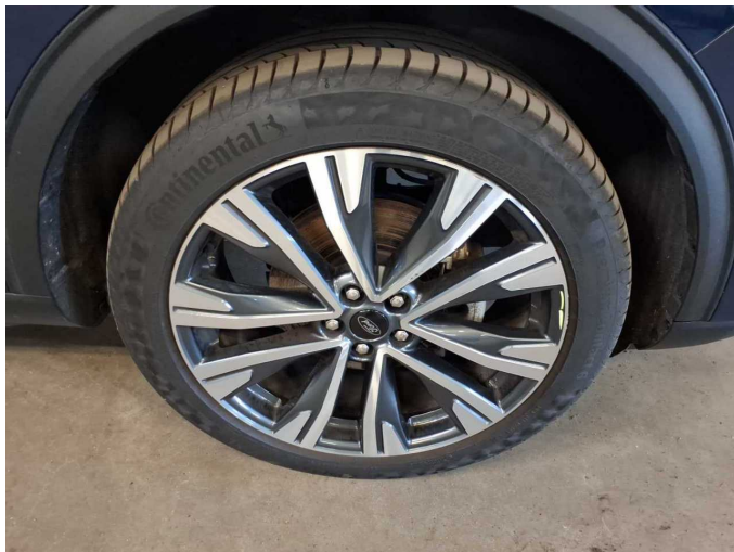
Damage 10: Wheel / tyres: Alloy rim - front right side (Materialabtrag) - Scratch(es) - Replace
