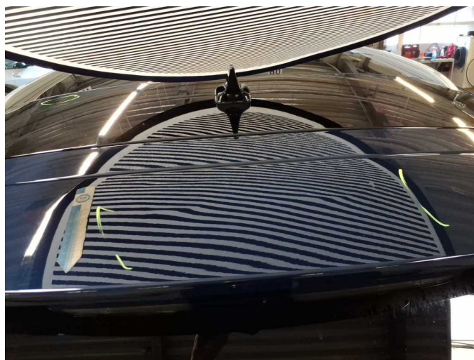
Wear and tear 4: Boot lid / rear door: Rear spoiler - dent(s)
