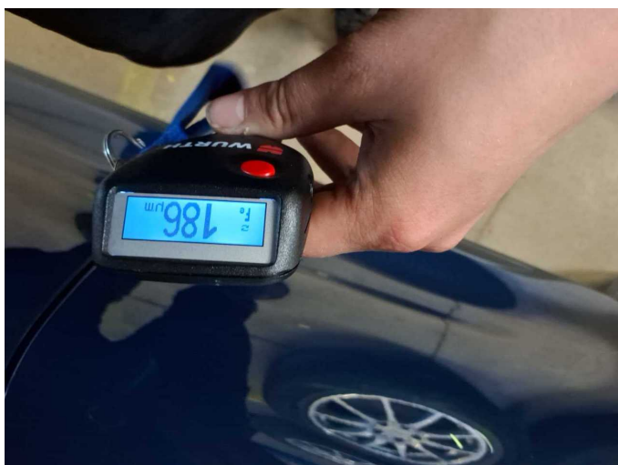
Roof rail - right side: 186 µm
