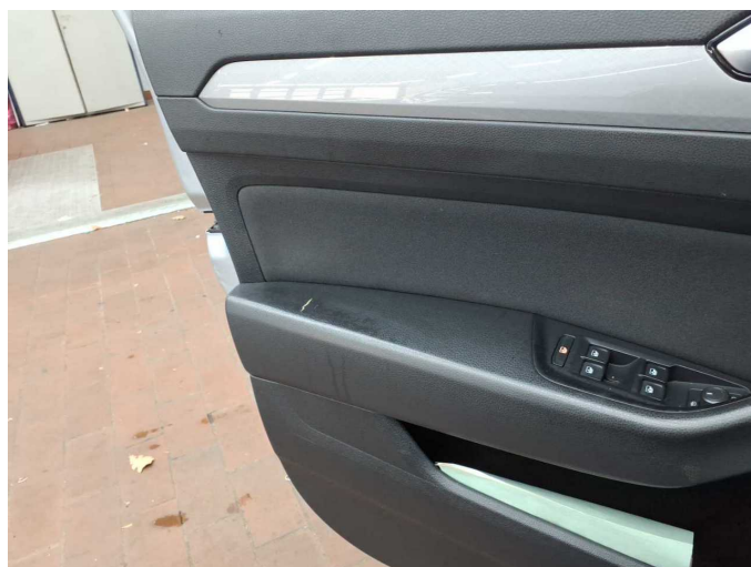
Damage 2: Trim / covers: Door trim - front left side (Armauflage) - Broken / torn - Replace
