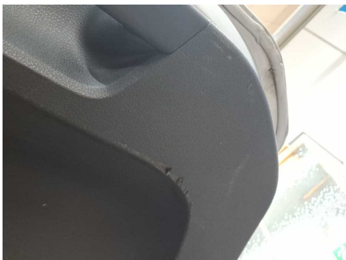
Damage 1: Interior: Interior - Scratch(es) - Loss in value
