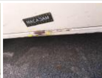
Outside rear-view mirror base L, Scratch(es), Replace
