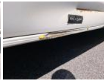
Sliding door R, Dent(s), Repair and paint (complete)
